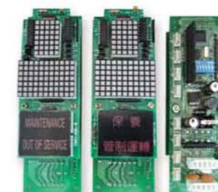
LAN Transmission Board Include Dot Matrix Hall Display
