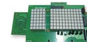
LAN Transmission Board Include Dot Matrix Car Display (Horizontal)
