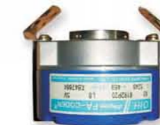
Encoder Tamagawa, Voltage: DC 5V Type:01H60-8192P20-L6-5V
